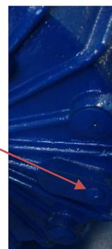
When the two plugs are removed screw the two brake release screws (42).
